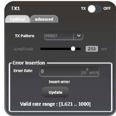
Figure 17: TX OFF - channel control locked
